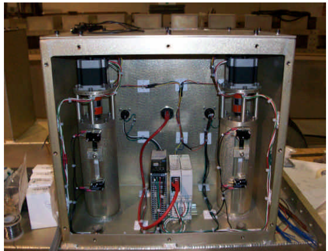
Ethernet Network-Connected Auto-Tuner
